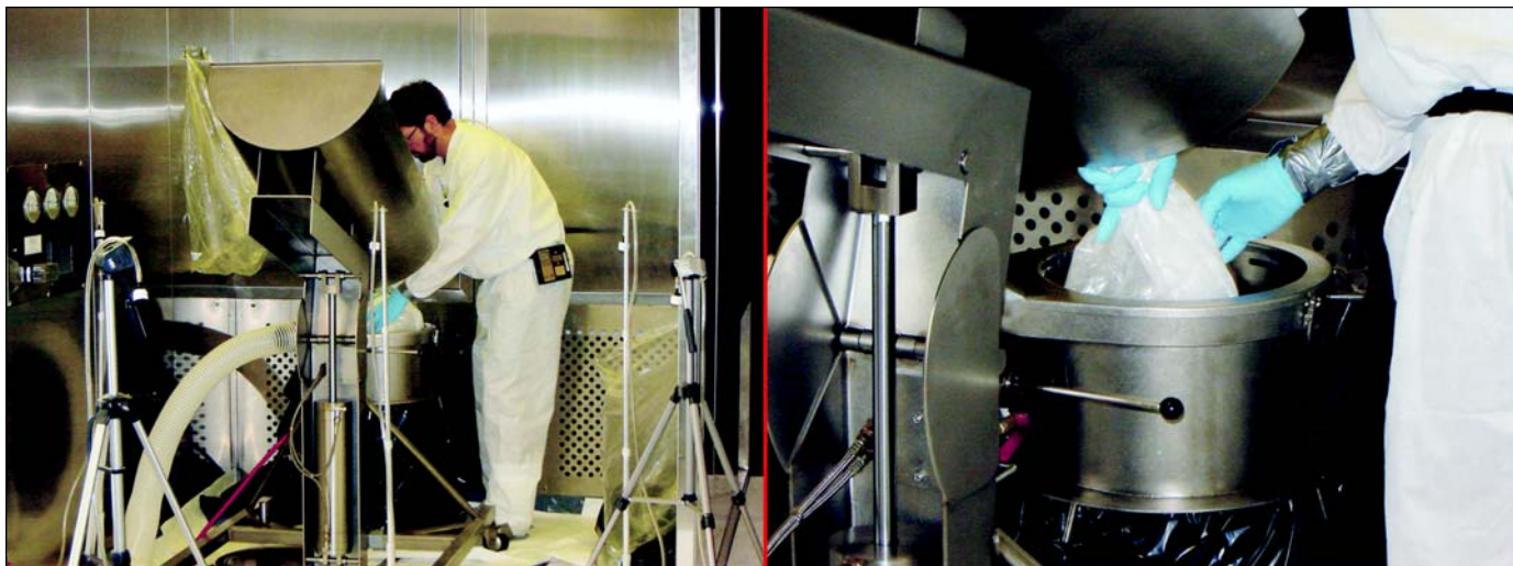
Figure 4. Lactose transfer from bulk drum by 'massaging' the contents slowly through the liner into the receiving drum.
